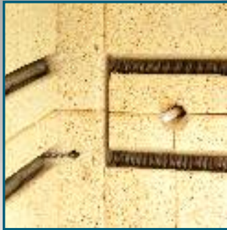
Platin-Rhodium-Thermoelement zur Temperaturerfassung - verschleißfrei sowie bruchgeschützt montiert Platinum-Rhodium-Thermocouple for temperature recording - free of wear as well as protected against break
